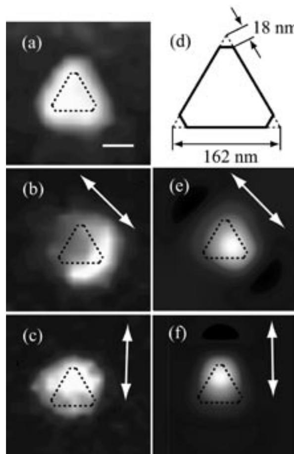
**Figure 1.** (a) Topography of a single gold triangle. (b), (c) Observed incident-polarization dependent TPI-PL images of the single gold triangle. (d) Schematic drawing of a snipped triangle used for calculations (e), (f). (e), (f) Calculated polarization-dependent electric field distributions near the snipped triangle. Arrows indicate the direction of the incident polarization. Dashed lines indicate approximate shape of the triangle. Scale bar: 100 nm.
