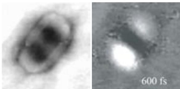
**Figure 1.** Typical near-field static transmission (left) and transient transmission change (right) images of gold nanorod (diameter 30 nm, length 300 nm). In the right panel, bleached and induced extinctions are indicated, respectively, in black and white.
