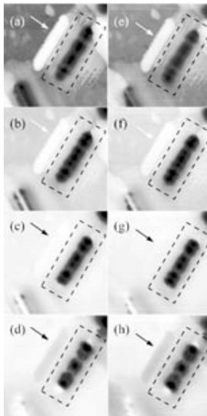
**Figure 1.** Transmission near-field optical images of a single gold nanorod (diameter  $22 \pm 3\text{ nm}$ , length  $510 \pm 30\text{ nm}$ ): (a–d) I-mode, (e–h) C-mode. The scan area is  $1\text{ }\mu\text{m} \times 1\text{ }\mu\text{m}$ . Observed spectral region: (a,e) 607–627 nm, (b,f) 647–666 nm, (c,g) 666–686 nm, (d,h) 705–725 nm. Arrows indicate *z*-motion artifacts.
