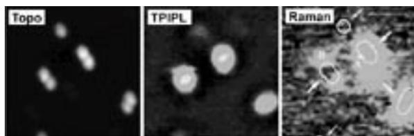
**Figure 1.** Topograph (left), near-field two-photon excitation (center), and near-field Raman excitation (right) images of gold nanospheres doped with R6G molecules. The Raman image was obtained for the R6G band at  $1340\text{ cm}^{-1}$ . Image size:  $1.5\text{ }\mu\text{m} \times 1.5\text{ }\mu\text{m}$ .
