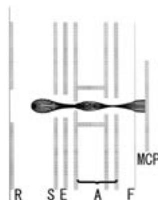
**Figure 1.** Schematic view of the threshold photoelectron spectrometer and simulated trajectories at the initial kinetic energy of 10 meV. From ionization center 36 electron trajectories were generated in the ejection angle of  $0^\circ$  to  $360^\circ$ , at an interval of  $10^\circ$ . R, repeller; S, screening electrode; E, extraction electrode; A, asymmetric lens system; F, front-plate electrode.
