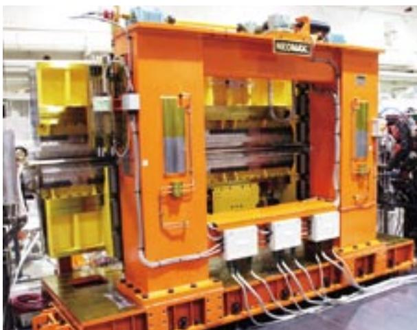
**Figure 1.** New variable polarization undulator for BL7U.
