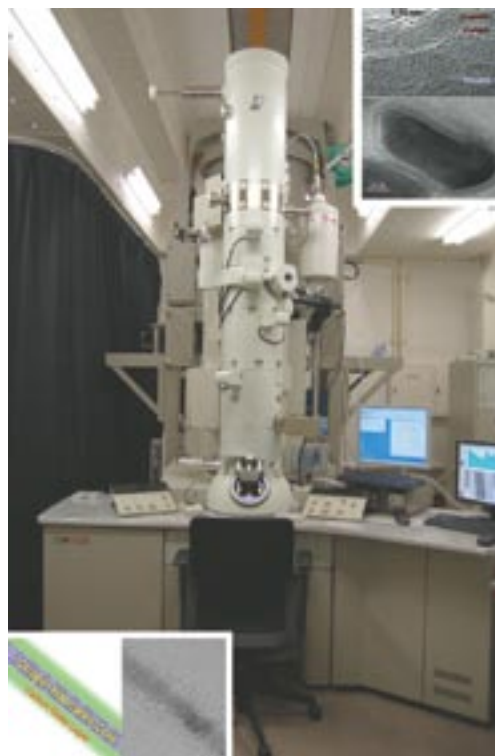
300kV Transmission Electron Microscopy and Some Typical Examples.
