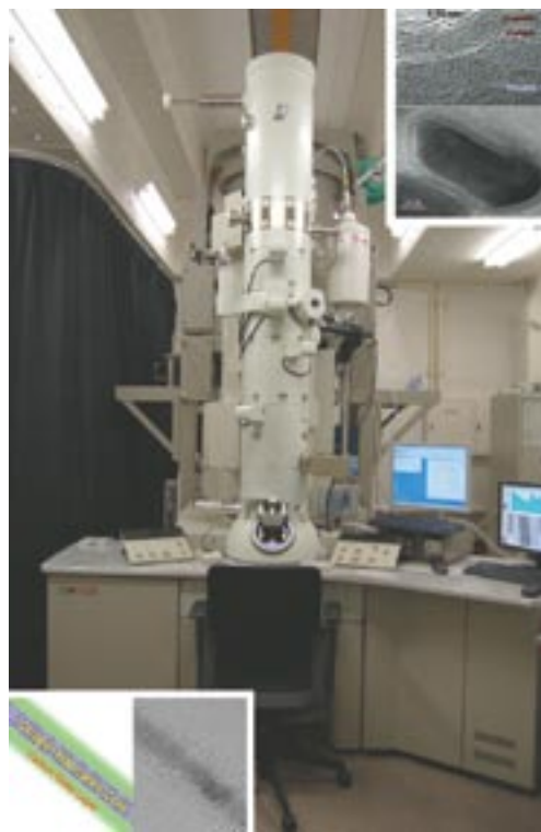
300kV Transmission Electron Microscopy and Some Typical Examples.
