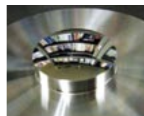
Figure 3. The 28mm diameter, surface-of-a-sphere with R60mm made by sending speed 10 micrometer/rev, spindle rotation speed 20 rpm, the vibration radius 2 micrometers and vibration frequency 39 kHz.
