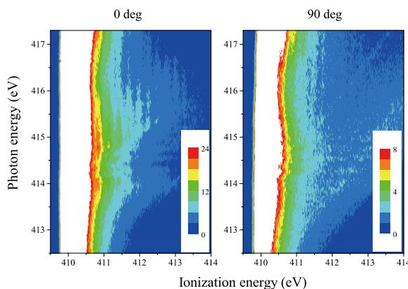
**Figure 2.** Two-dimensional maps of the inner-shell photoelectron yields from  $\text{N}_2$  as a function of photon energy and ionization energy, measured in the photon energy region of 412.5–417.3 eV at (a) 0° and (b) 90° with respect to the electric vector.
