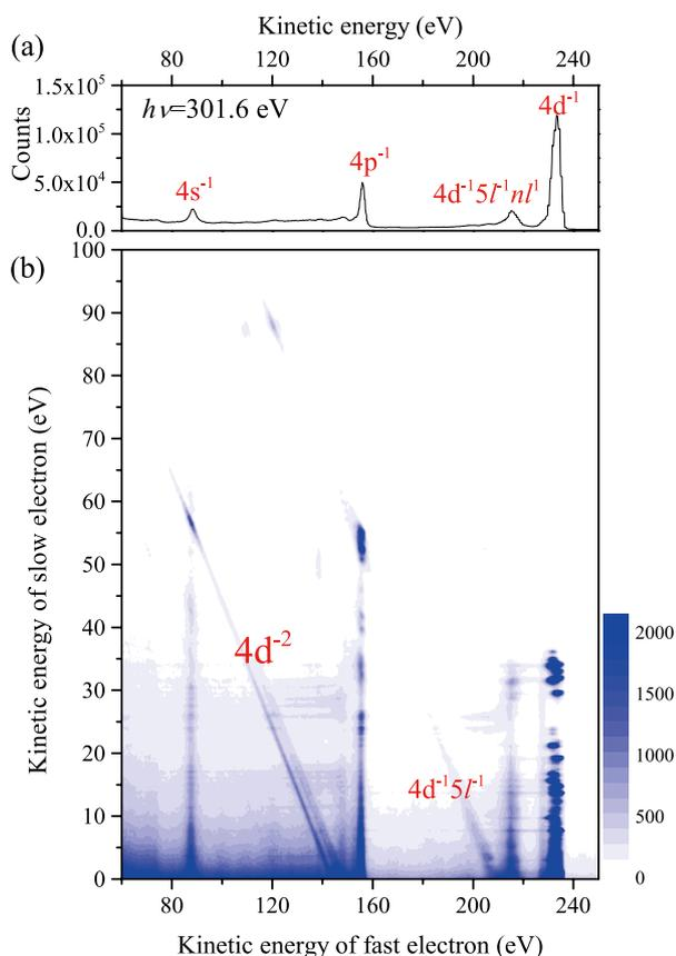
**Figure 1.** (a) Photoelectron spectrum of Xe obtained at a photon energy of 301.6 eV. (b) Two dimensional map of all coincidence pairs, represented as a function of the kinetic energies of fast and slow electrons.
