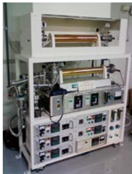
Figure 1. Photograph of single-crystal formed sublimation apparatus.
