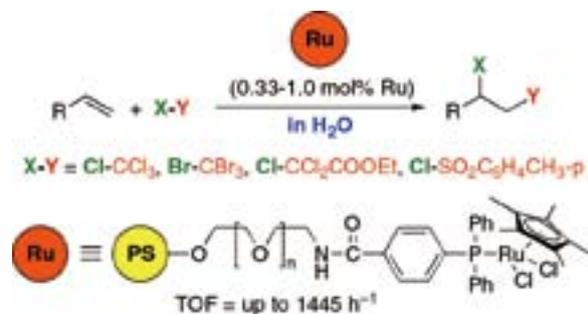
**Scheme 4.** Kharasch Reaction in Water with an Amphiphilic Resin-Supported Ruthenium Complex.
