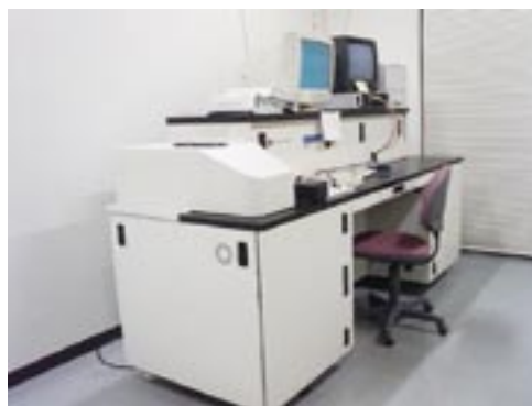
Figure 2. Matrix-Assisted Laser Desorption Ionization—Time of Flight Mass Spectrometer (Applied Biosystems Voyager DE-STR).
