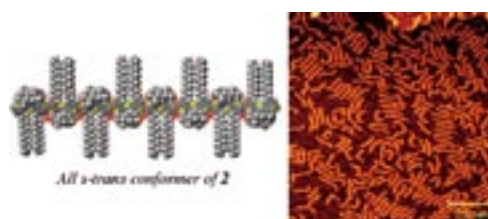
Figure 2. Structure of oligomer ( 2 ) and Large-area STM image.
