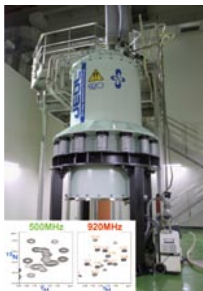
Figure 1. 920 MHz NMR spectrometer and an example measured using 920 and 500 MHz spectrometers. Much higher resolution in 920 MHz can be clearly seen.
