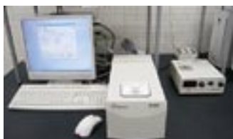
Figure 1. Differential scanning calorimeter (VP-DSC).
