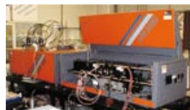
Figure 5. Excimer+dye laser (Lambda physics LPX 105i + LPD3002)
