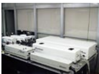
Figure 1. Differential scanning calorimeter (VP-DSC).
