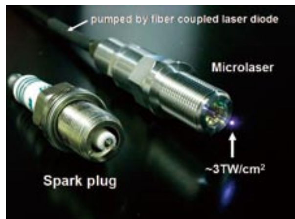
Figure 2. First prototype micro-laser module (right), which has the same dimension as a spark plug (left).
