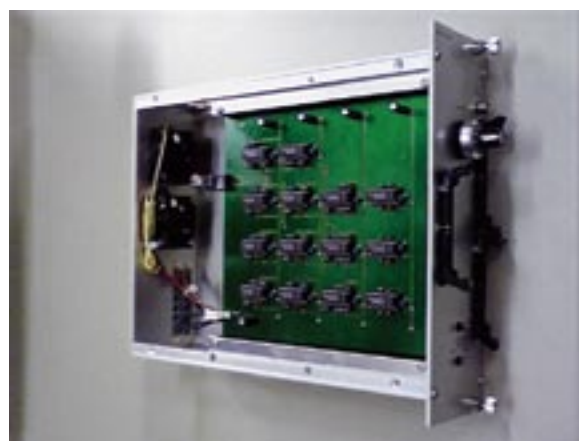
Figure 1. The multi-coincidence electronic circuit.
