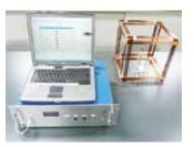
Figure 1. Magnetic field compensation device.
