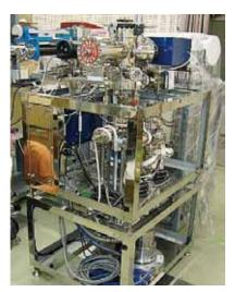
**Figure 2.** Photocathode Electron Gun to produce spin polarized electron beam.
