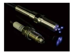
Figure 1. Microchip laser with three-beam output.
