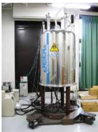
Figure 1. 600 MHz NMR spectrometer (JEOL JNM-ESA600).
