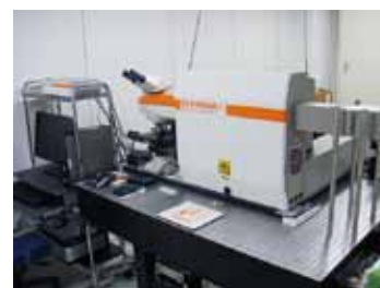
Figure 3. Raman microscope (Renishaw INVIA REFLEX532).
