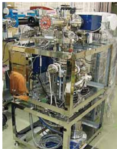
Figure 2. Photocathode Electron Gun to produce spin polarized electron beam.
