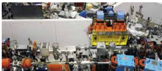
Figure 1. New APPLE-II type undulator just after the installation in spring, 2011. Another undulator will be installed in autumn 2011. Both of them will be used to produce coherent synchrotron radiation.
