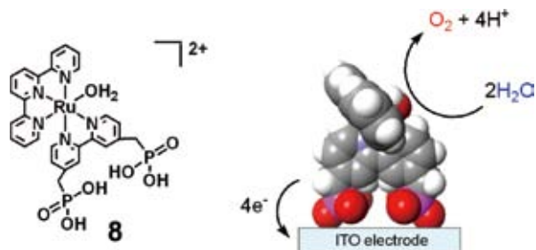
Figure 2. Schematic view of the electrochemical water oxidation catalyzed by a mononuclear ruthenium complex ( 8 ).
