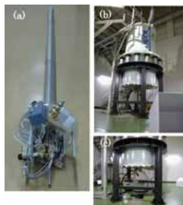
Figure 1. (a) The bottom view of newly developed VT-MAS probe. (b) The side view of VT-MAS probe loaded into 920 MHz ultra high field magnet (21.6 T). (c) The side view of VT-MAS probe and peripherals enabling VT.
