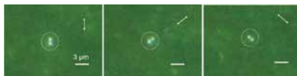
Figure 3. Two gold nanoparticles trapped by ultrashort pulses. Two particles are trapped separately and aligned along the incident laser polarization (arrows).
