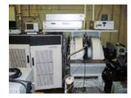
**Figure 2.** Pulse ESR for Q-band (Bruker E680).
