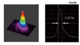
(a) Beam profile (b) Pulse duration Figure 1. Beam profile and pulse duration at 3.6 mJ.
