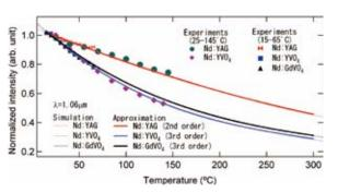
Figure 4. Temperature dependence of emission intensity of various Nd-doped laser media.
