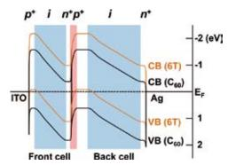
**Figure 5.** Energy structure of a tandem cell in real scale.  $n^+p^+$ -heavily doped homojunction acts as an ohmic interlayer connecting two single cells.
