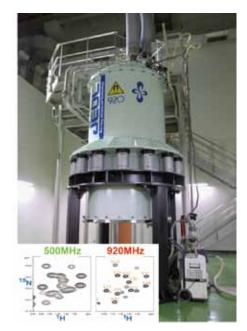
**Figure 1**. 920 MHz NMR spectrometer and an example measured using 920 and 500 MHz spectrometers. Much higher resolution in 920 MHz can be clearly seen.
