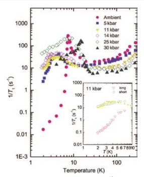
**Figure 1**. Temperature dependence of the <sup>13</sup>C-NMR spin-lattice relaxation rate,  $1/T_1$ , at six different pressures.
