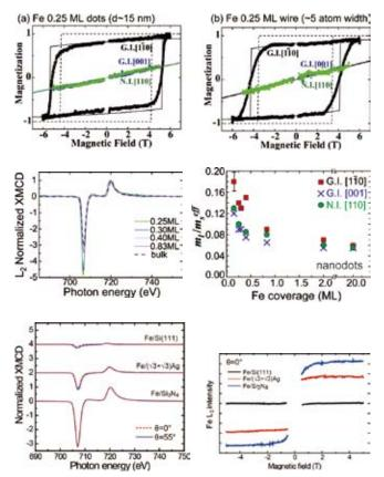
mated to be >15 T. Huge magnetic anisotropy can be concluded both for the nanodots and nanowires. By fitting the experimental data with a simple anisotropic magnetic energy model, the magnetic anisotropic constants were determined to be  $\sim$ 1 meV for both the in-plane and out-of-plane directions, which is a few hundred times larger than that of bulk *bcc* Fe.
