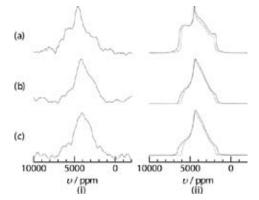
**Figure 3.**  $^{95}$ Mo NMR static spectra of {Mo<sub>12</sub>}(Ni) under the magnetic field of (a) 21.8 and (b, c) 11.7 T. (b) and (c) show the spectra at 301 and 173 K, respectively. (i) and (ii) show the observed and simulated spectra, respectively. The solid and broken lines in (ii) show the theoretical curves with and without considering the hyperfine interaction, respectively.
