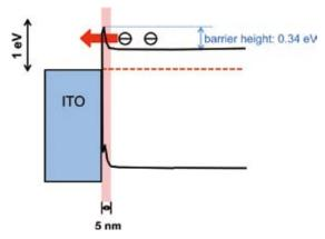
**Figure 3.** Energy structure for  $ITO/n^+$ -C<sub>60</sub> contact in real scale. A tunneling ohmic junction for photogenerated electrons is formed.
