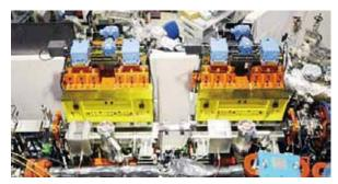
Figure 1. Variable Polarization Optical Klystron at UVSOR-III.
