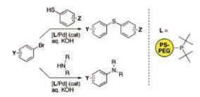
**Scheme 3.** C–N and C–S Bond Forming Cross Coupling in Water with Amphiphilic Resin-Supported Pd Complexes.
