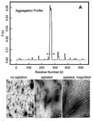
**Figure 1.** The aggregation profile of GroEL obtained by the analysis with PASTA (A), and the transmission electron microscopic observations of the isolated apical domain at pH 7.0 and 37 °C at 0.1 M NaCl in the presence of 0.5 mM SDS, where the amyloid-like fibrils of the apical domain were formed when the solution was agitated.
