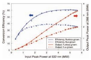
Figure 2. FHG conversion characteristics by different BBO crystal.
