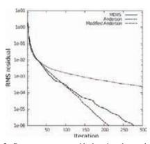
**Figure 2.** Root mean square residual against the number of iteration steps for the calculation of 3D site distribution profiles of water around a DNA molecule by 3D-RISM. Solid, dotted, and dashed lines are for MDIIS, Anderson, and Modified Anderson algorithms, respectively.
