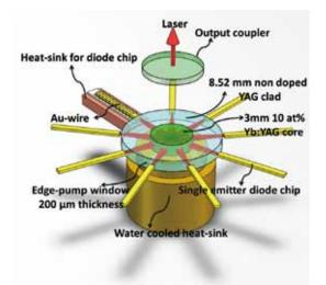
Figure 3. The scheme of lens-less edge-pumped microchip laser.
