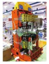
**Figure 2.** New Undulators installed in 2011. The upper is the variable polarization optical klystron undulator which will be used for coherent light generation. The lower is the in-vacuum undulator for the STXM beam-line.
