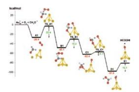
**Figure 4.** Energy diagram of reaction pathway I in the aerobic oxidation of methanol to formic acid on  $Au_{20}^{-}$  (kcal/mol).
