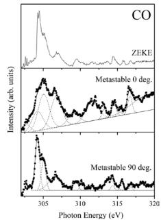
**Figure 2.** ZEKE spectrum, and angle-resolved metastable yield spectra, measured at  $0^{\circ}$  ( $\Sigma$ -symmetry) and  $90^{\circ}$  ( $\Pi$ -symmetry), in the satellite and double/triple excitation regions of CO in the C *K*-edge region.
