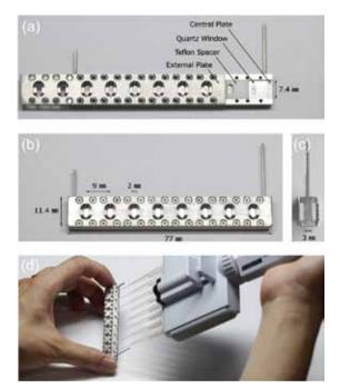
**Figure 2.** Octuple cuvette. (a) Photograph of the central plate covered by the quartz window, Teflon spacer and external plate, in that order. (b) Front view of the assembly. (c) Side view of the assembly. (d) Filling and removal of solutions using a commercially available eight-channel pipette. The sample volume of each chamber is  $25 \,\mu$ l.
