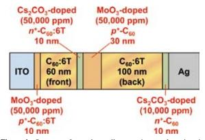
Figure 4. Structure of a tandem cell connecting two homojunction cells, which is made only by doping to  $C_{60}$ :6T codeposited film.
