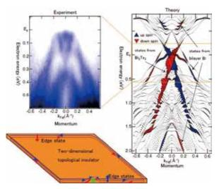
**Figure 3.** The experimental band dispersion of Bi(111) bilayer on  $Bi_2Te_3$  measured experimentally (left) and its corresponding first-principles calculations (right). The left bottom figure shows the schematic drawing of a two-dimensional topological insulator.
