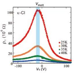
**Figure 3.** Gate voltage dependence of the resistance for  $\kappa$ -Cl based Mott-FET. Because this device clearly shows ambipolar behavior due to a smaller number of mid-gap trap states, it is possible to exactly define the gate voltage for charge neutrality point ( $V_{\text{Mott}}$ ). This fact helps determining the critical exponent for Mott transition, which is important both for theoretical investigation and for analyzing device parameters such as subthreshold swing.
