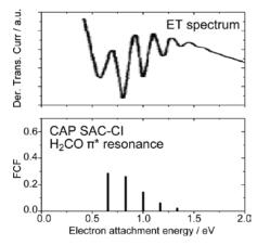
**Figure 2.** Vibrational structure in  $\pi^*$  resonance of H<sub>2</sub>CO by the projected CAP/SAC-CI method compared with the electron transmission spectrum.
