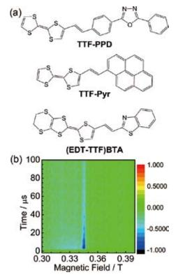
**Figure 2.** (a) Molecular structure of single-molecule-type photoconductive materials, TTF and EDT-TTF derivatives. (b) 2D pulsed TR-ESR spectra for powder sample of photoconductive EDT-TTF containing BTA. The normal axis represents the ESR signal intensity. The color scale denotes the signal intensity. Positive and negative values indicate the absorption and emission of microwaves, respectively.
