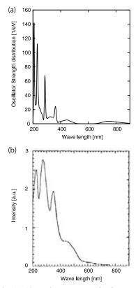
**Figure 1.** (a) Absorption spectrum of a face-centered cubic unit associated with a solid thin film of  $C_{60}$  in comparison with (b) the experimental observation.
