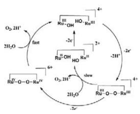
Scheme 3. Four-electron oxidation of water catalyzed by  $[Ru^{III}_2(OH)_2(bpy)_2(btpyan)]^{4+}$ .
