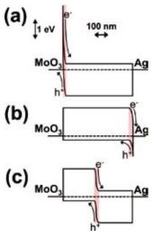
**Figure 2.** Energy structures for  $Cs_2CO_3$ -doped (a), MoO\_3-doped (b), and  $Cs_2CO_3$ -/MoO\_3-doped (c) cells in real scale based on the Kelvin probe measurements. Photocarrier generation occurs in the depletion regions (shaded).
