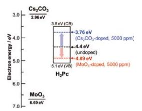
**Figure 1.** Energy diagram of a H<sub>2</sub>Pc film. The broken lines show the energy levels of  $E_{\rm F}$  for undoped (black), MoO<sub>3</sub>-doped (red) and Cs<sub>2</sub>CO<sub>3</sub>-doped (blue) H<sub>2</sub>Pc films.
