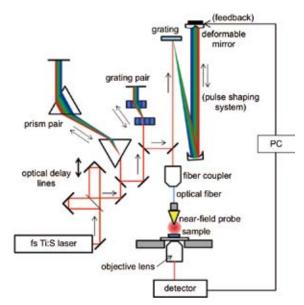
Figure 2. Experimental setup of sub-20-fs ultrafast near-field measurement.
