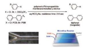
**Scheme 2.** Instantaneous Hydrodehalogenation of Haloarenes by a Microflow Device Containing a Polymeric Pd Nanoparticles Membrane.
