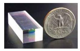
Figure 5. 10-mm-thick PPMgLN device with QPM period  $\Lambda = 32.2 \ \mu m$ .
