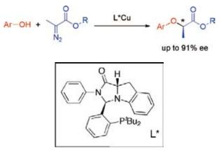
**Scheme 4.** Enantioselective Carbenoid Insertion into Phenolic O–H Bonds with a Chiral Copper(I) Imidazoindolephosphine Complex.
