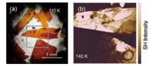
**Figure 1.** (a) Thin crystals of  $\alpha$ '-(BEDT-TTF)<sub>2</sub>IBr<sub>2</sub> in a sapphireanvil cell loaded with liquid argon. (b) SHG image in the square region of (a) (T = 140 K).
