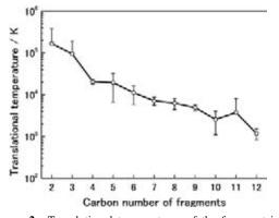
**Figure 2.** Translational temperatures of the fragment ions from coronene at hv = 100 eV. Error bars show the standard deviations of repeated experimental runs.
