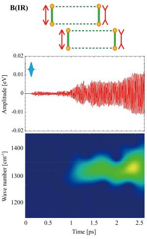
**Figure 1.** C=C stretching phonon mode B (infrared active) schematically represented in the upper panel. Its time evolution (middle panel) and time-frequency spectrogram (lower panel) on the initially neutral dimer are shown when the charge-separated state is photoexcited.
