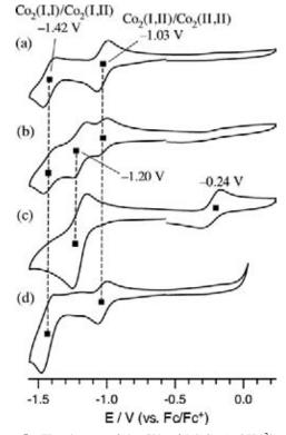
**Figure 5.** The changes of the CVs of  $[(1)Co_2(\mu-OH)]^{3+}$  with the addition of CF<sub>3</sub>SO<sub>3</sub>H (a) 0 eq., (b) 1.0 eq., (c) 2.0 eq. and (d) after the addition of 5 eq. *i*PrNEt<sub>2</sub>.
