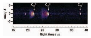
**Figure 1.** *Y*–*t* map of parent and fragment ions produced from  $C_{70}$  with the excitation *hv* of 110 eV. The *y* coordinate is proportional to the *y* component of the ion velocity.
