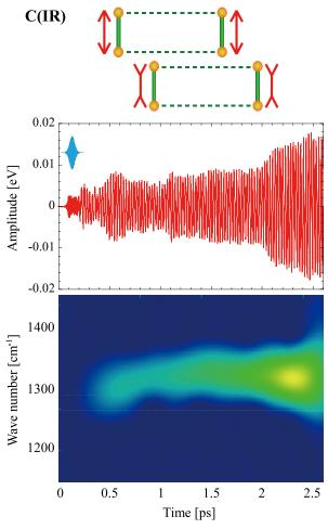
**Figure 2.** C=C stretching phonon mode C (infrared active) schematically represented in the upper panel. Its time evolution (middle panel) and time-frequency spectrogram (lower panel) on the initially neutral dimer are shown when the charge-separated state is photoexcited.
