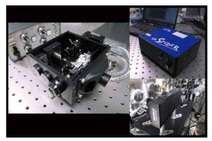
**Figure 1.** (left) A Fringe-Resolved Autocorrelation (FRAC) apparatus for sub-10 fs pulse characterization designed in the Center. (upper right) Spectral Phase Interferometry for Direct Electric-Field Reconstruction (SPIDER) and (lower right) Frequency-Resolved Optical Gating (FROG) apparatuses for general-purpose ultrashort pulse characterization.
