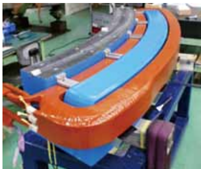
Figure 1. New combined function bending magnet (a lower half is shown).
