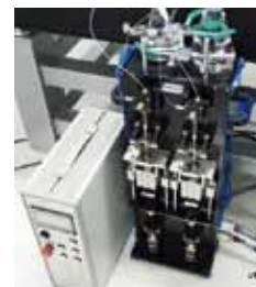
Figure 1. Picture of the rapid buffer-exchange system.
