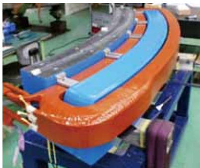
Figure 1. New combined function bending magnet (a lower half is shown).
