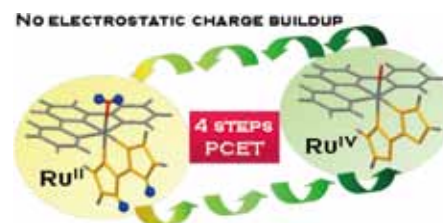
Figure 1. A schematic view of the four-step PCET reaction of 1 to give the four-electron oxidized species, [Ru^{IV}(trpy)(bim)(O)]^{2+} .
