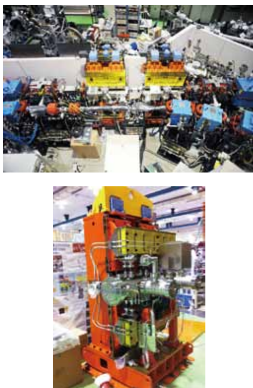
Figure 2. New Undulators installed in 2011. The upper is the variable polarization optical klystron undulator which will be used for coherent light generation. The lower is the in-vacuum undulator for the STXM beam-line.
