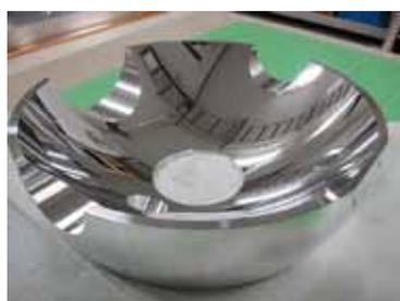
Figure 1. Ellipsoidal Reflector for Inverse Photoelectron Spectroscopy.
