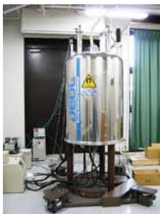
**Figure 1.** 600 MHz NMR spectrometer (JEOL JNM-ECA600).
