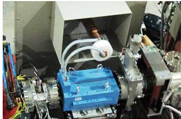
Figure 1. Pulse sextupole magnet developed for UVSOR-III.
