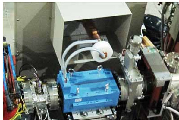
Figure 1. Pulse sextupole magnet developed for UVSOR-III.
