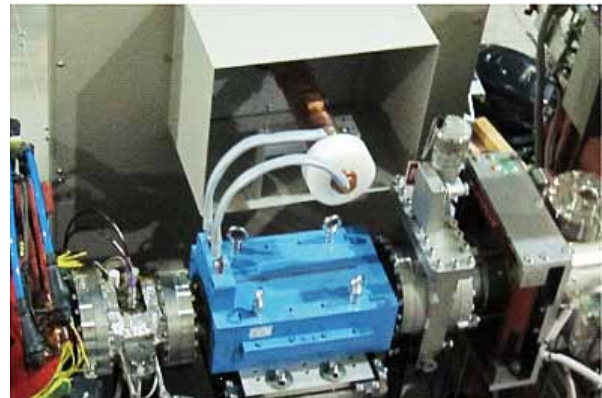
Figure 1. Pulse sextupole magnet developed for UVSOR-III.
