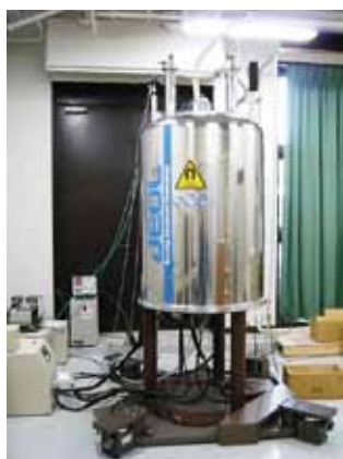
Figure 1. 600 MHz NMR spectrometer (JEOL JNM-ECA600).
