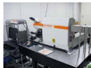
Figure 3. Raman microscope (Renishaw INVIA REFLEX532).
