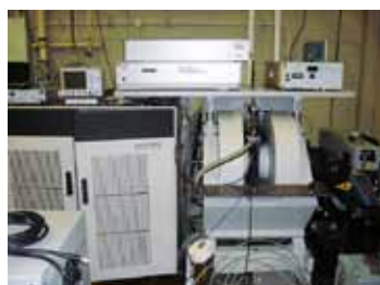
Figure 2. Pulse ESR for Q-band (Bruker E680).
