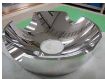
Figure 1. Ellipsoidal Reflector for Inverse Photoelectron Spectroscopy.
