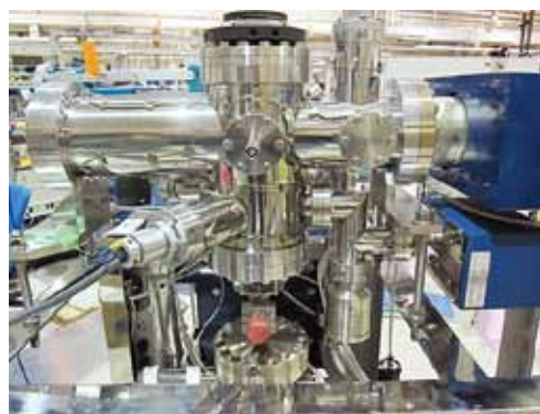
Figure 1. Spin polarized electron gun under commissioning at UVSOR.
