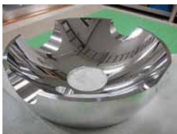
Figure 1. Ellipsoidal Reflector for Inverse Photoelectron Spectroscopy.
