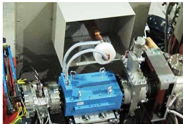
Figure 1. Pulse sextupole magnet developed for UVSOR-III.
