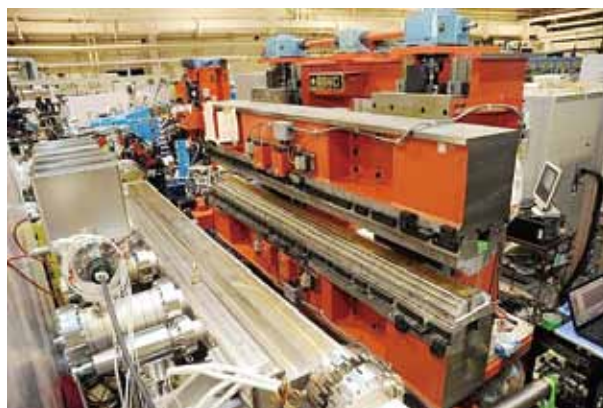
Figure 3. Remodeling of Variable Polarization Undulator at BL5U.
