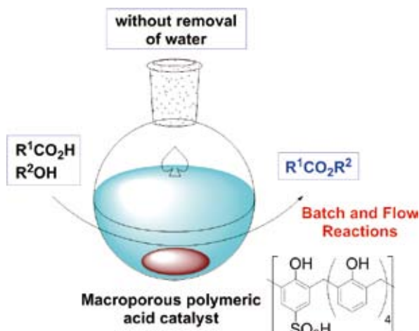
Figure 3. Direct dehydrative esterification of alcohols and carboxylic acids with a macroporous polymeric acid catalyst.
