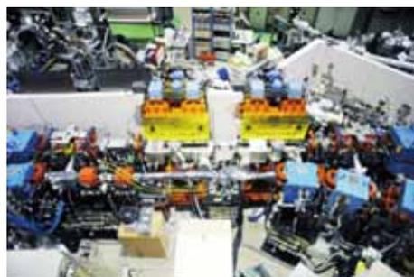
Figure 1. Twin Polarization-variable Undulator System at UVSOR-III.
