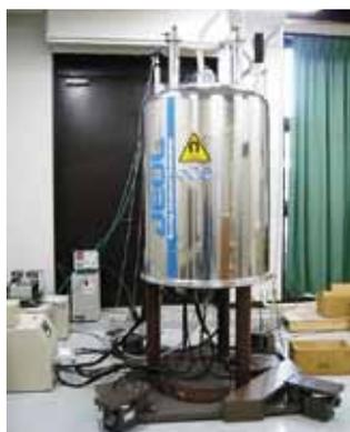
**Figure 1.** 600 MHz NMR spectrometer (JEOL JNM-ECA600).
