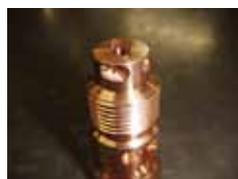
**Figure 3.** Cathode plug for electron emission.
