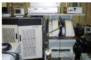
Figure 2. Pulse ESR for Q-band (Bruker E680).
