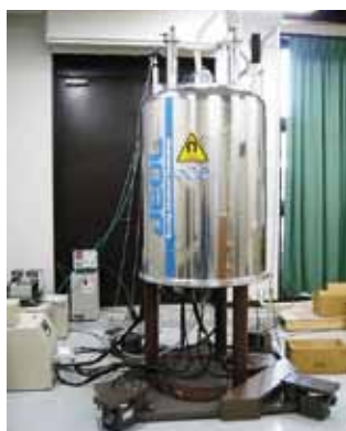
Figure 1. 600 MHz NMR spectrometer (JEOL JNM-ESA600).
