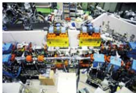
Figure 1. Twin Polarization-variable Undulator System at UVSOR-III.
