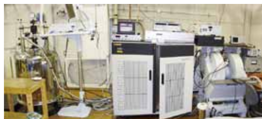
Figure 1. Solid state broad-line NMR system (above). Multi-frequency pulsed ESR system (below).
