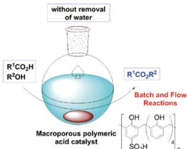
Figure 3. Direct dehydrative esterification of alcohols and carboxylic acids with a macroporous polymeric acid catalyst.
