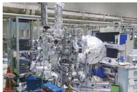
Figure 2. Picture of the new spin-resolved ARPES end station of BL5U, UVSOR-III.
