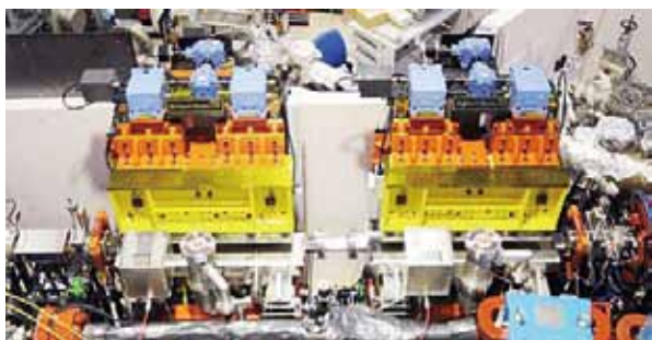
Figure 2. Twin Polarization-variable Undulators for Coherent Synchrotron Radiation generation.
