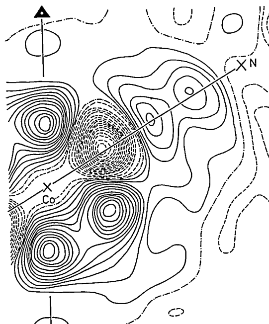
Figure 1. Section of the difference Fourier map through a Co-N bond and a C_3 axis. Contours are at intervals of 0.05 \text{ e}\text{\AA}^{-3} . Negative contours are dotted, and zero being chain-dotted. Resolution: 2\sin\theta_{\max}/\lambda = 1.81 \text{ \AA}^{-1} .
