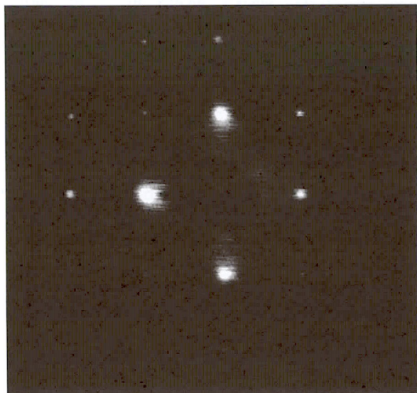
Figure 1. The LEED image of NaCl(100) surface on the Ge(100)(2x1) surface. The thickness of the film is estimated to be 30 ML.
