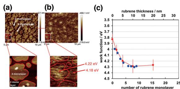
**Figure 5.** (a) Morphological image of Mo<sub>3</sub>O<sub>9</sub> (1,000 ppm) doped homoepitaxial rubrene having the thickness of 5 nm. (b) Simultaneously obtained potential image. Magnified image (lower) of white rectangle area (upper) are also shown. Island shapes emphasized by red curves are overlaid in the potential image. (c) Monolayer-digitized band mapping.
